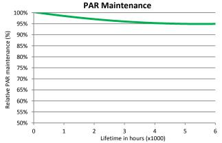
Ushio Hi-LuxGro AMH-DE1000W/AGRO the trend line is based on tests under defined and stable laboratory conditions and represents an average of all values measured.
