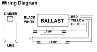
The wiring diagram that appears above is for the lamp type denoted by the asterisk  $(\ensuremath{^*})$
