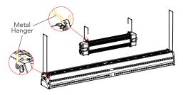
• Next mount the driver using the S shaped metal hangers provided on the same beam.
